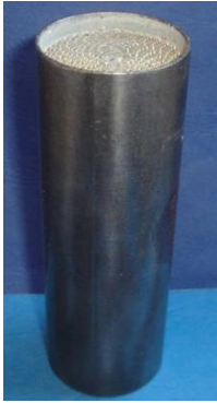
Figure 18 Honeycomb methanation reactor (Buchholz, 2015).
